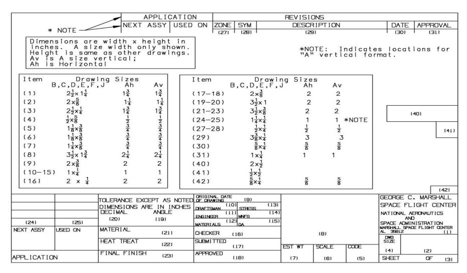
FIGURE 2. DRAWING FORMAT BLOCK SIZES (Not to Scale)
