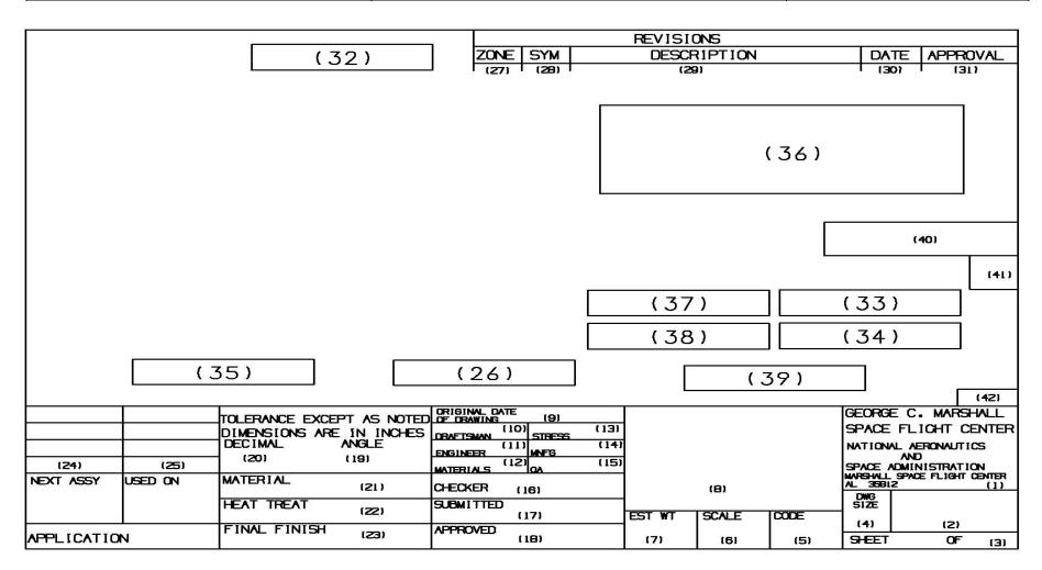
FIGURE 1. DRAWING FORMAT (Not to Scale)
