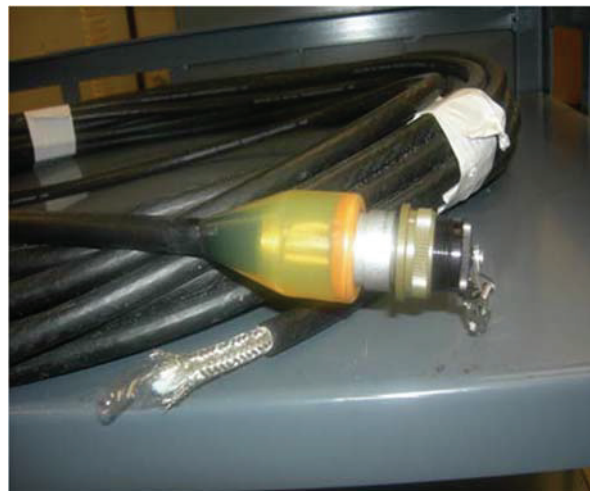
Figure 12. Typical Cable Assembly Showing One End Terminated
