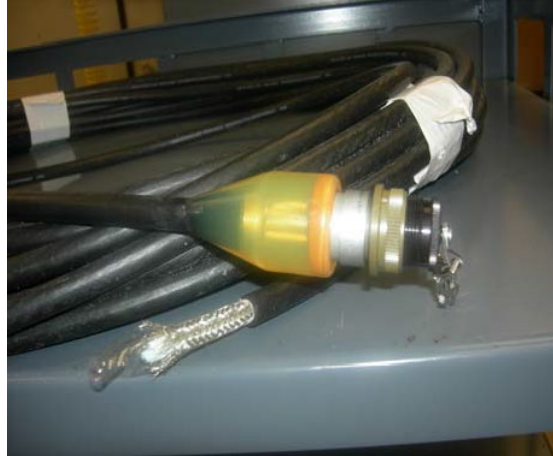
Figure 5. Typical Cable Assembly Showing One End Terminated
