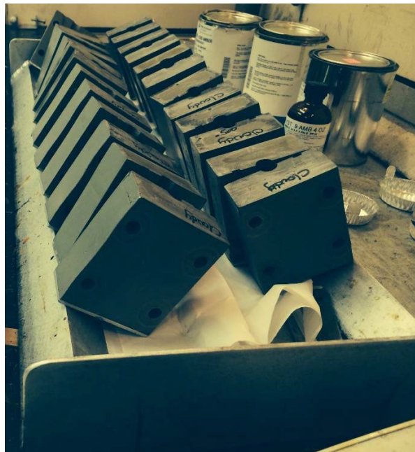
Figure 6. Drip Table/Rack and Tilted Mold Boxes for Releasing Entrained Air
