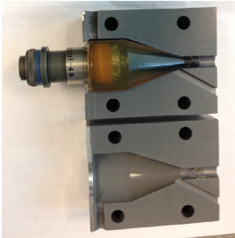
Figure 11. Completed Mold Halves with Completed Cable Assembly End
