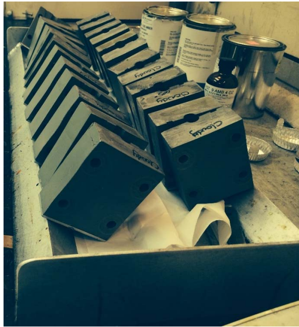
Figure 13. Drip Table/Rack and Tilted Mold Boxes for Releasing Entrained Air
