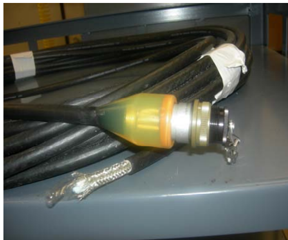
Figure 12. Typical Cable Assembly Showing One End Terminated
