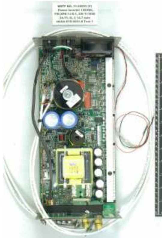
b. Internal view, case removed after test
