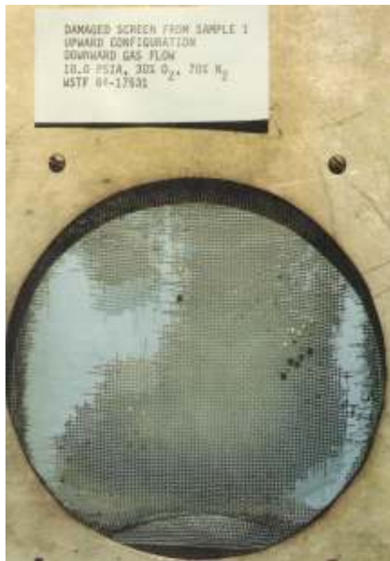
Figure 11. Damaged Aluminum Vent Screen from Airflow Tests
