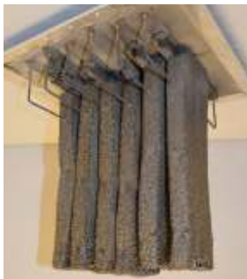
c. Posttest (burned foam -- 80% free volume, 20% foam)
